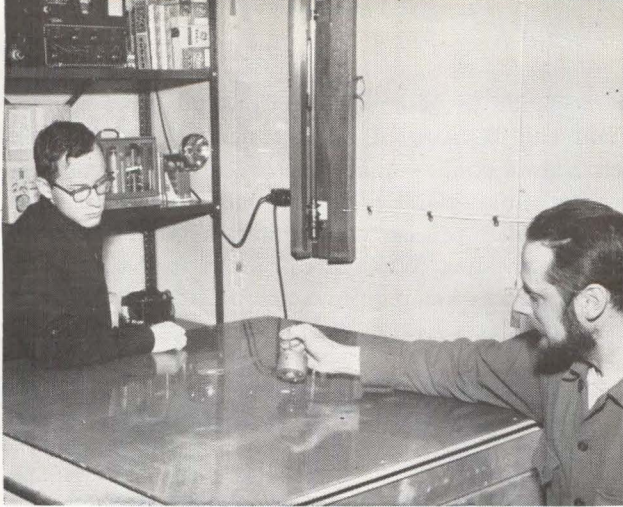
RADIO ACTIVE radium element is placed in cosmic ray neutron monitor pile at Bartol Research Foundation's Antarctica base
