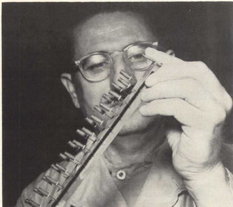
TANTALUM capacitors have been made more reliable by close control of all production operations
