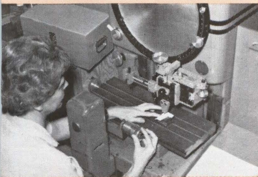
Inspection at magnifications up to 50 times, with tracer for contoured surfaces.
