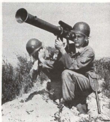
TILT, a device that shoots infrared beams instead of bazooka shells, keeps score in war games. It was developed by Raytheon
