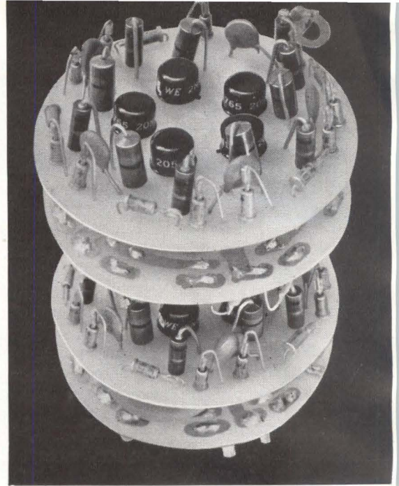
MODULES in 8-Kv experimental switch assembly are mounted back to back to limit inductance
