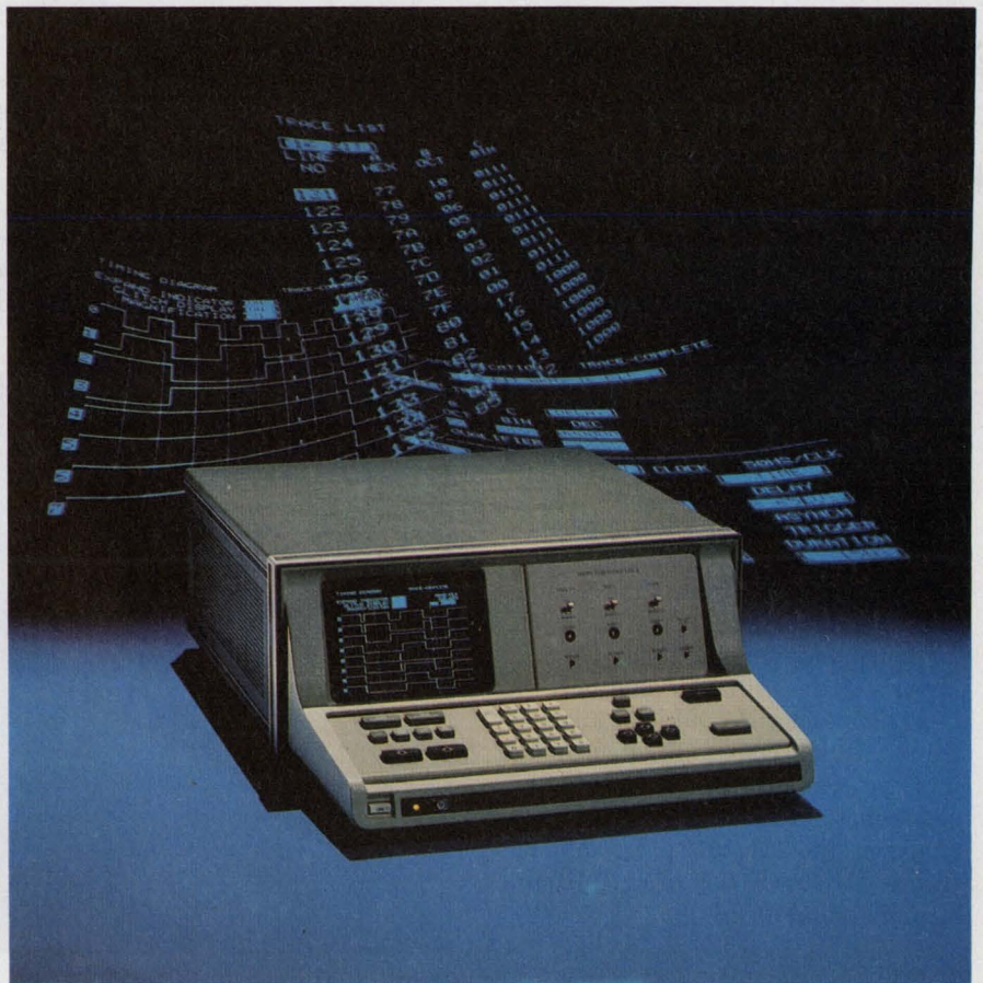
Timing or state analysis, or both at the same time, is a feature of Hewlett-Packard's Model 1615A. It can also catch glitches as short as 5 ns, and display them on a built-in CRT. Price is $6800.
