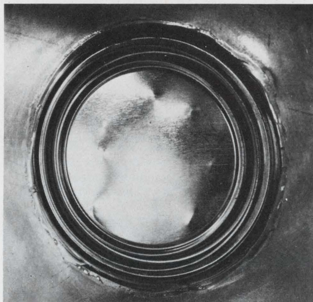
1. A paint-can lid installed in a test panel is an example of a good rf seam design.
