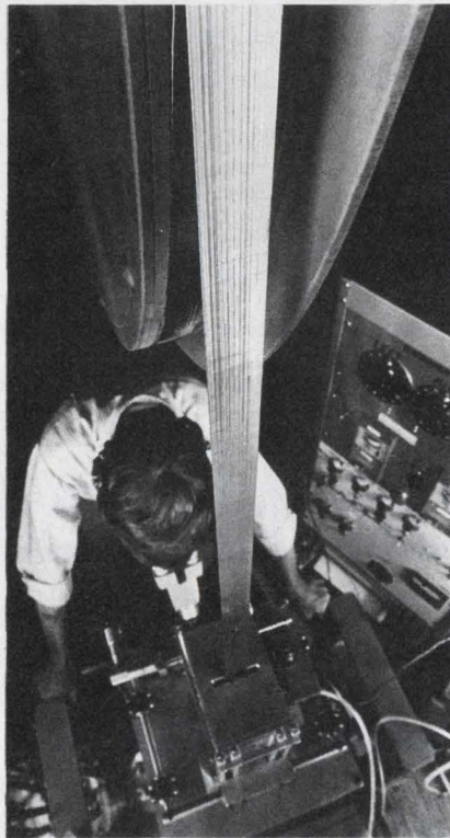
1. Long continuous ribbons of silicon crystal grown at Mobil Tyco Labs may lead to mass-produced low-cost solar cell arrays.
