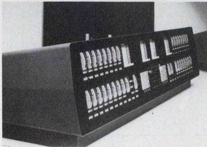
The TDC 2000 Total Distributed Control system made by Honeywell (1100 Virginia Dr., Fort Washington, PA 19034. 215-643-1300) integrates  $\mu$ P-based controllers, stand-alone CRT display stations and a data bus for information transfer. It can be combined with process computer hardware and software packages to provide the flexibility for controlling processes ranging from the most simple to the most advanced.
