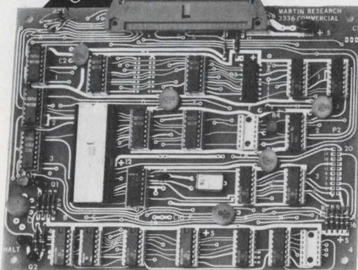
The **MIKE 3** is a good example of the flexibility of the **modular micro** approach. An optimal small system — yet fully expandable. A three-board version, the AT813, includes the Model 471 CPU board (with 8080A); memory board with 8080 Monitor PROM, 512 bytes RAM (expandable to 2K PROM, 1K RAM); console board with keyboard, six LED digits; connectors; and Manual . . . only \$395. (Manual alone, \$35.) Priced at \$149. in quantities of one, with 8080A, the 471 CPU features:
