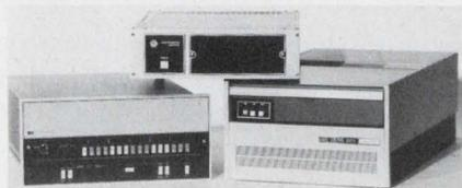
The MSM-10X high density disc-storage system made by Microcomputer Systems Corp. (3068 Kenneth St., Santa Clara, CA 95050. 408-985-1414) can store up to 225 million bytes. It uses a microprogrammed controller that is totally integrated with the host computer's operating system. The disc system can transfer data at a 1.2 Mbyte/s rate and can support up to four disc drives
