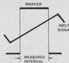
doing with your input waveform. Use the markers on the second channel of your scope to see where the counter is triggering. Really useful thanks to the 5328A's 100 MHz ECL outputs. Standard.
