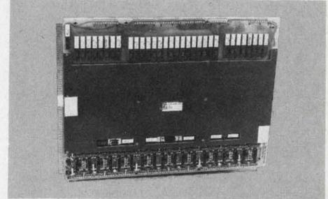
**16K/32K Memory Systems.** Model 696: 16K, 18-bits; to 256K X 9, 128K X 18, 64K X 36. Model 698: 32K, 18 bits; to 512K X 9, 256K X 18, 128K X 36. Cycle 650 nsec, access 250 nsec. Dir. rplcmnts for Micro 3000. Fabri-Tek, Inc., 5901 S. Cnty. Rd. 18, Mpls, MN 55436 (612) 935-8811
