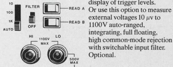
Or use this option to measure external voltages 10  $\mu$ v to 1100V auto-ranged, integrating, full floating, high common-mode rejection with switchable input filter. Optional.
