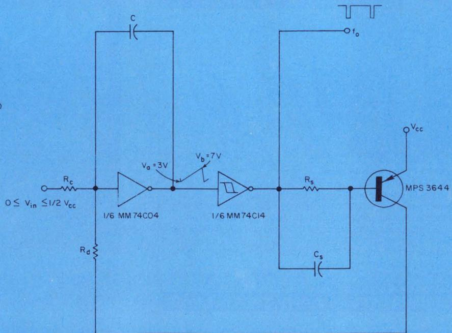
The frequency output of this VCO varies linearly from a 5.5-kHz maximum, when the control voltage
