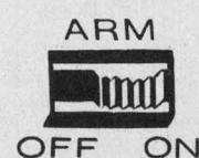
The counter goes to work when your command tells it to. Ideal for burst frequency or sweep generator linearity measurements. Standard.
