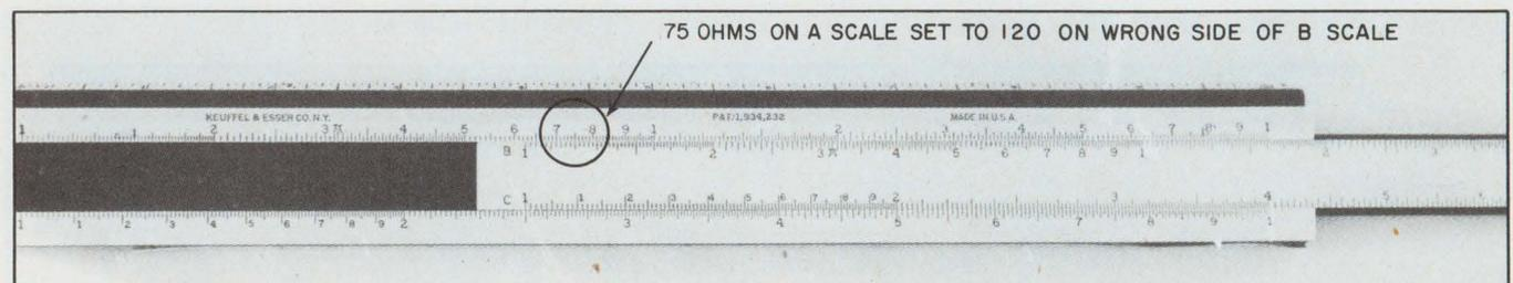
12. An incorrect turns ratio will appear if the wrong half of the A or B is used.
