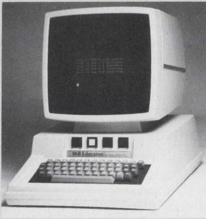
The M-8 Educator development system, designed by Technical Communications Inc. (P.O. Box 306, Olathe, KS 66061. 913-764-0243), provides a CRT communications terminal and  $\mu$ P controller in one unit. The system is built around the Fairchild F-8 microprocessor and includes a 53-key (Hall-Effect) keyboard, 64-character-by-31-line CRT display, 110-baud TTY-compatible serial I/O, 300 or 600-baud TTL serial I/O, composite video output signal for remote CRT and 2-k of RAM, expandable to 32-k.
