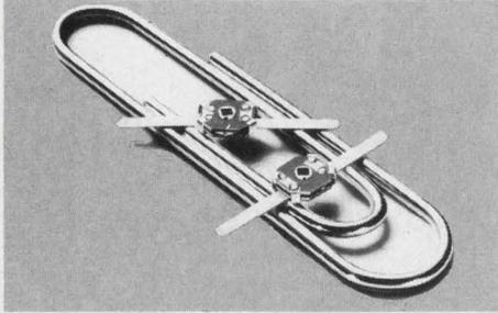
**Thin-Trim variable capacitors** provide a reliable means of adjusting capacitance without abrasive trimming or interchange of fixed capacitors. Series 9401 has high Q's and a range of capacitance values from 0.2-0.6 pf to 3.0-12.0 pf and 250 WVDC working voltage. Johanson Manufacturing Corporation, Boonton, New Jersey (201) 334-2676.
