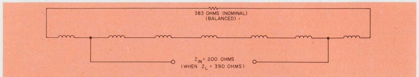
11. A seven-winding autotransformer is needed to match 383 to 200 Ω, both balanced to ground.
