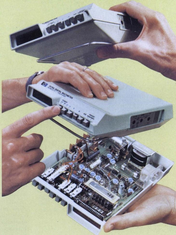
Tantalum nitride on sapphire processing allows replacement of all front end precision resistors by a single chip. That means greater reliability and better temperature stability. Of course it's input protected.
