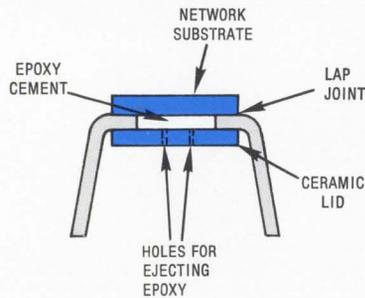
Various types of DIP packaging are utilized of which the molded and "sandwich" types seem most common. One problem that frequently occurs with the sandwich types is delaminating. This happens when air in tiny voids remaining in the epoxy filler (bonds the substrate to the sandwich "lid") expands in hot operating environments to the extent that the package comes apart and fails.
