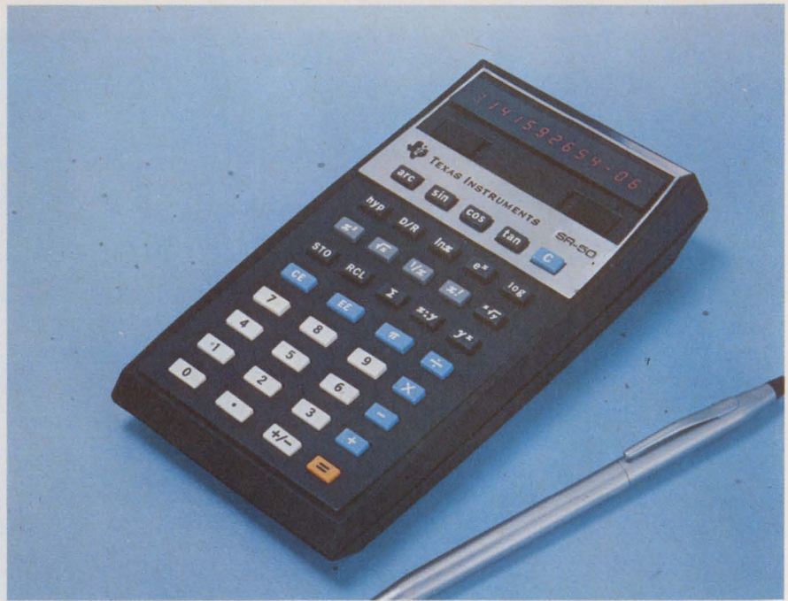
Over 53 independent-key functions are provided by this TI SR-50 calculator. Arithmetic of this unit is organized as hierarchic algebra.
