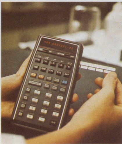
The only pocket-sized calculator with programming capability, the HP-65, uses magnetic-strip cards containing up to 100 program steps.
