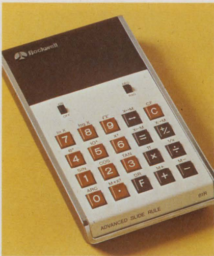
Capabilities of this eight-digit, floating-point calculator, the Rockwell 61R, are duplicated in a sizable number of other machines.
