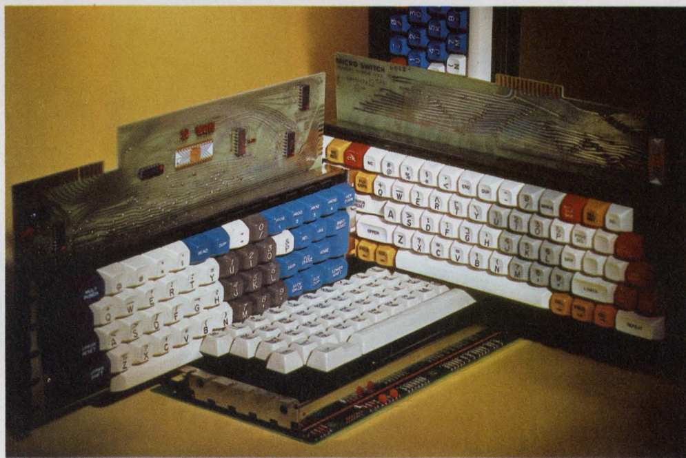
Micro Switch's line is represented by these MOS and TTL-encoded data-preparation and communications keyboards. Each uses the Hall-effect keyswitch.
