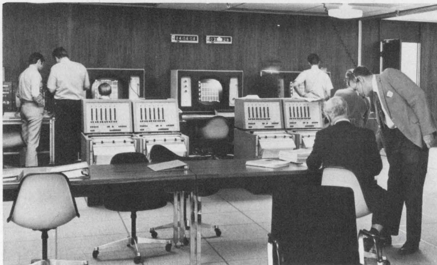
Telemetry systems at the Atlantic Fleet Weapons Range in Puerto Rico receive signals from missiles being fired by the fleet in practice drills.
