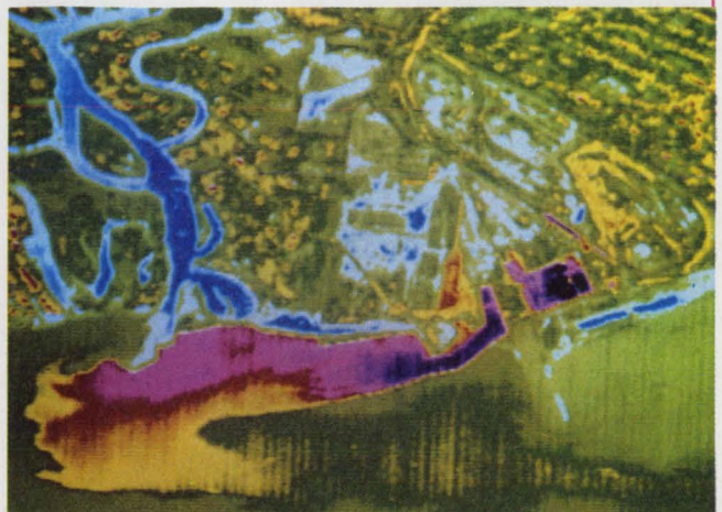
yellow and green are cool), the isothermal contours of the waterway become evident and the thermal pollution of the waterway can be analyzed.
