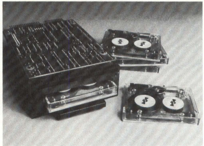
Figure 5: Irwin Magnetics' model 210 tape drive is the first to use DC100A-class minicartridges in a 3 1/2" Winchester footprint. Interface is floppy compatible.
