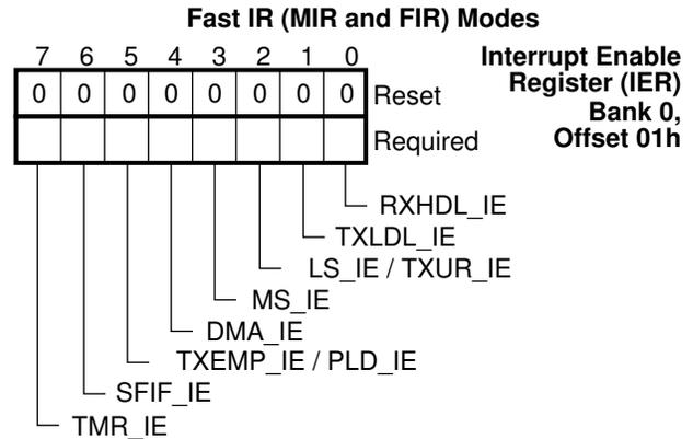
**FIGURE 5-8. IER Register Bitmap, MIR and FIR Modes**
