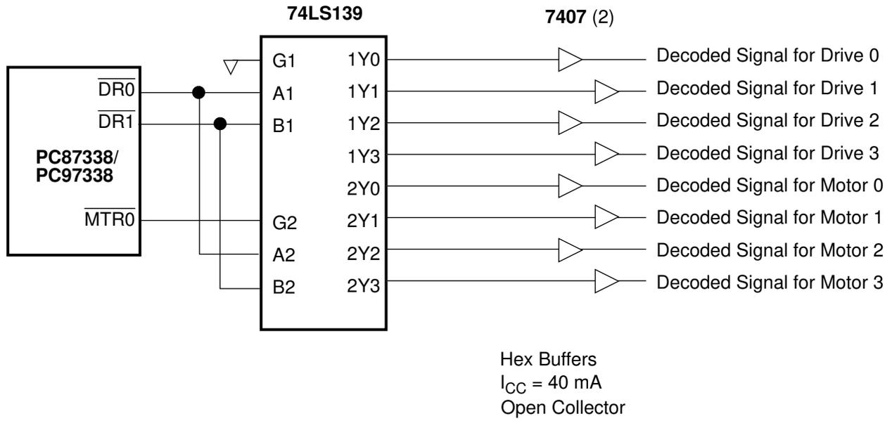
**FIGURE 3-19. PC87338/PC97338 Four Floppy Disk Drive Circuit**
