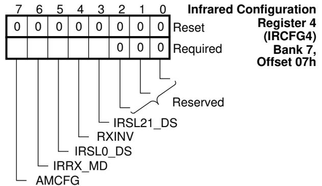
**FIGURE 5-56. IRCFG4 Register Bitmap**
