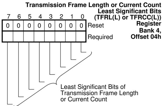
**FIGURE 5-36. TFRL(L) or TFRCC(L) Register Bitmap**
