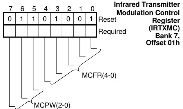
**FIGURE 5-51. IRTXMC Register Bitmap**
