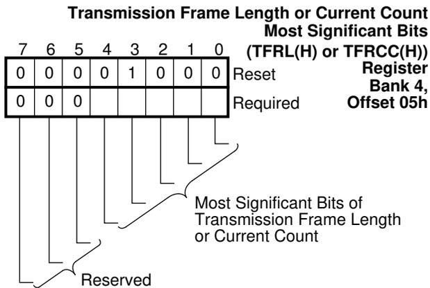
**FIGURE 5-37. TFRL(H) or TFRCC(H) Register Bitmap**
