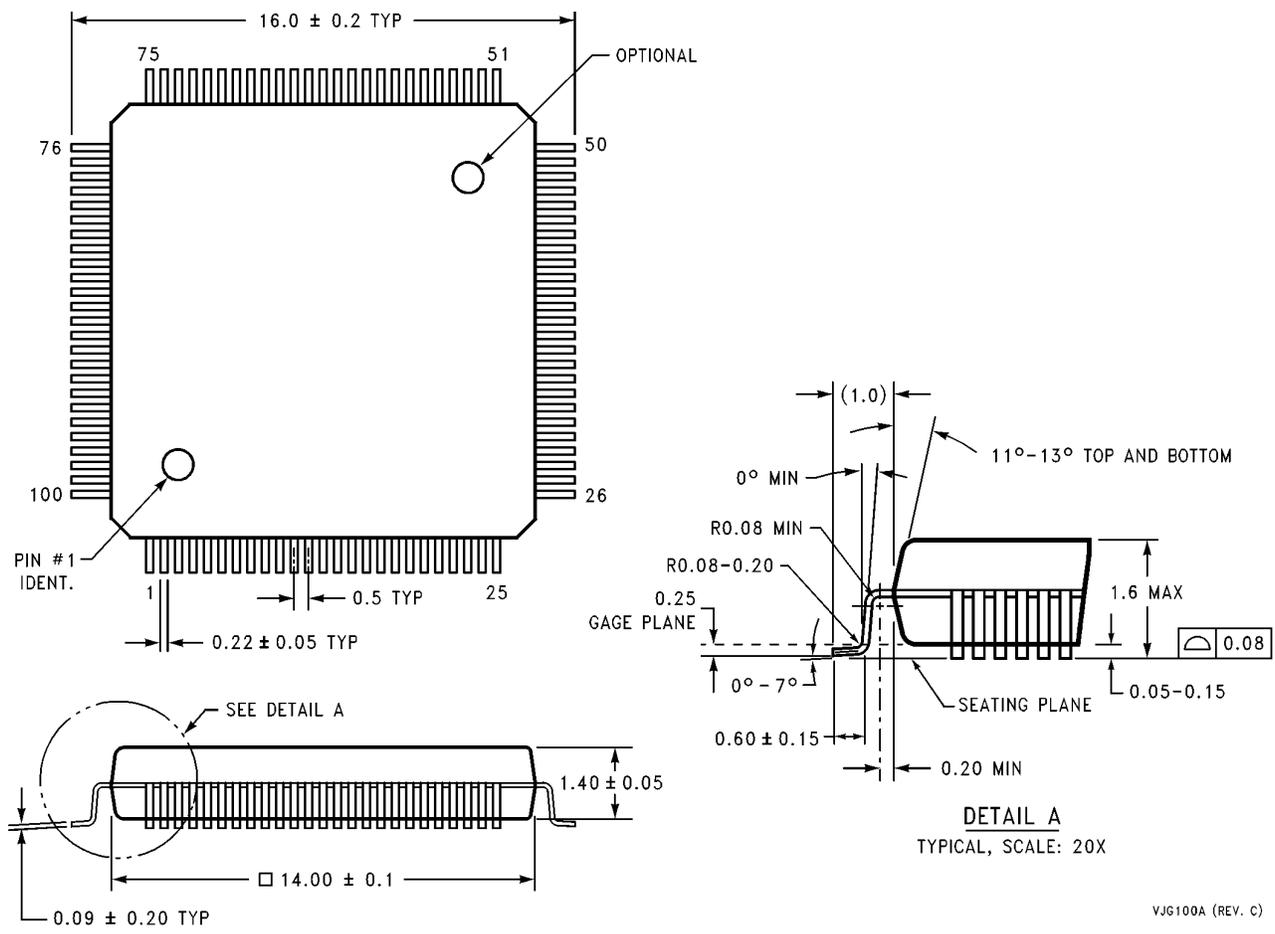
Thin Quad Flatpack (TQFP), JEDEC
