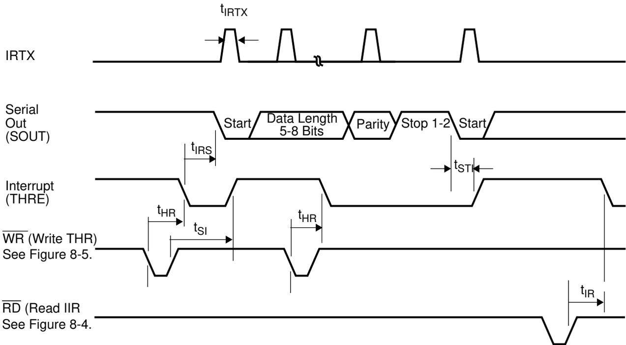
**FIGURE 8-8. SIR Transmitter Timing**
