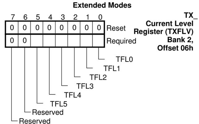
**FIGURE 5-28. TXFLV Register Bitmap**
