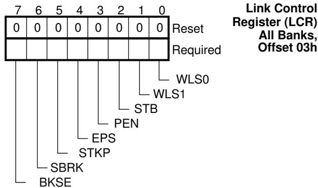
**FIGURE 5-13. LCR Register Bitmap**
