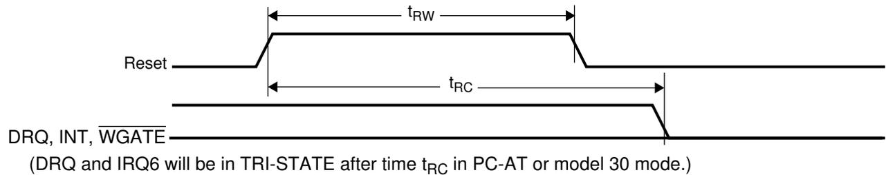
**FIGURE 8-18. Reset Timing**
