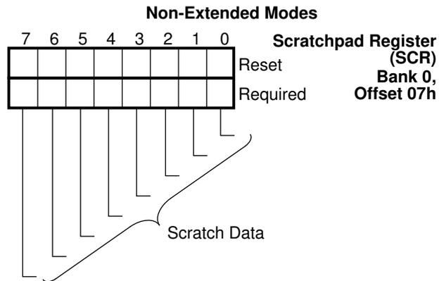
FIGURE 5-19. SPR Register Bitmap
