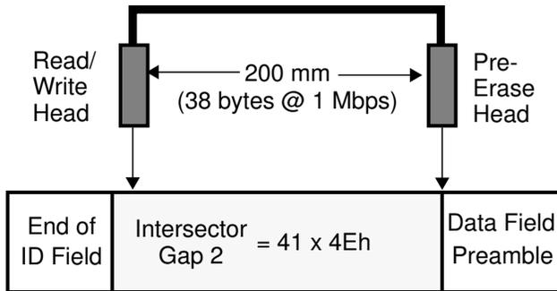
**FIGURE 3-4. Perpendicular Recording Drive Read/Write Head and Pre-Erase Head**
