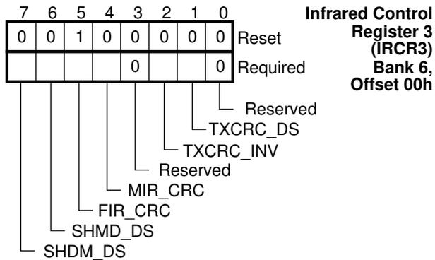
**FIGURE 5-46. IRCR3 Register Bitmap**
