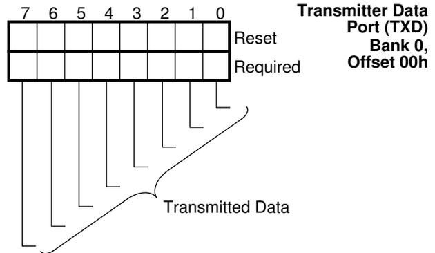
**FIGURE 5-4. TXD Register Bitmap**
