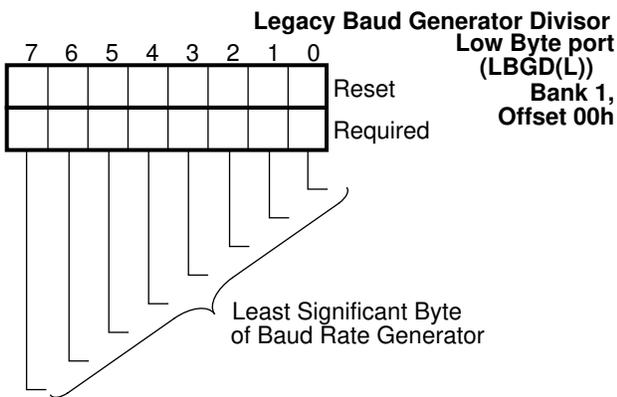
**FIGURE 5-21. LBGD(L) Register Bitmap**
