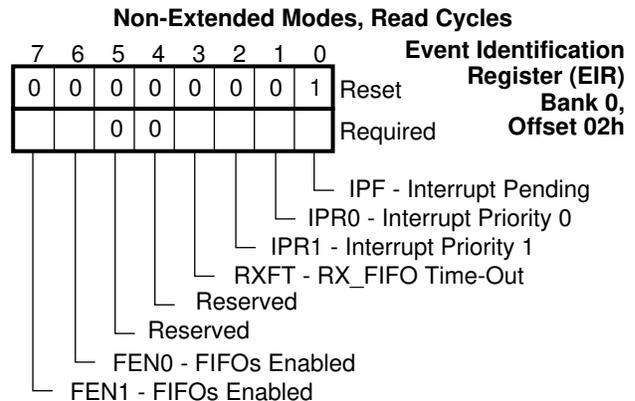
**FIGURE 5-10. EIR Register Bitmap, Non-Extended Modes**
