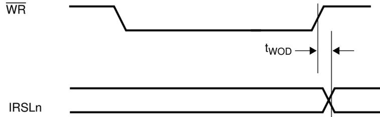
FIGURE 8-15. IRSLn Write Timing
