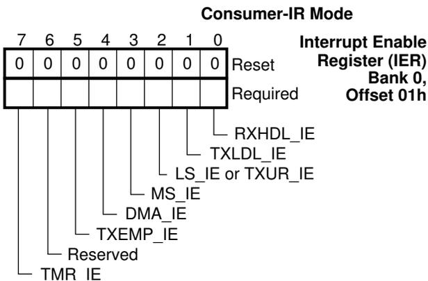
**FIGURE 5-9. IER Register Bitmap, Consumer-IR Mode**
