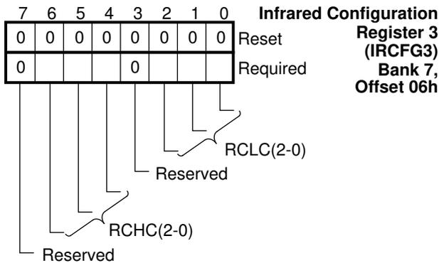
**FIGURE 5-55. IRCFG3 Register Bitmap**
