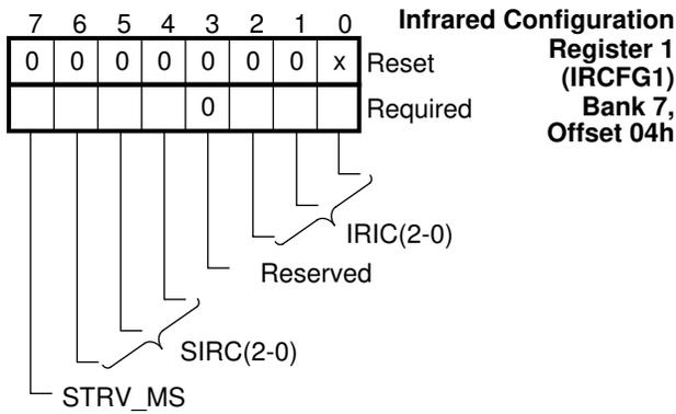
**FIGURE 5-53. IRCFG1 Register Bitmap**
