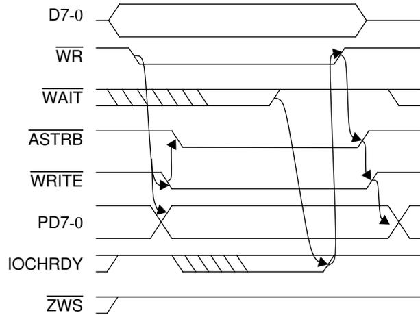
**FIGURE 4-13. EPP 1.7 Address Write**
