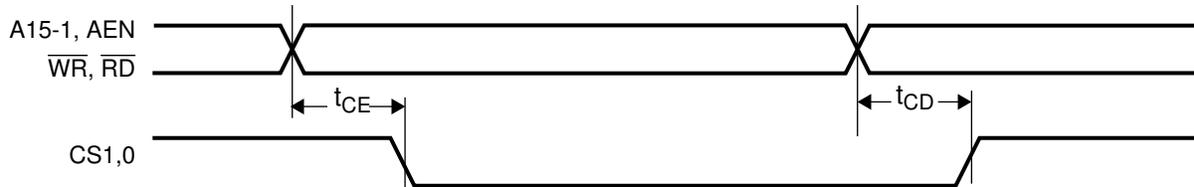
FIGURE 8-30. Chip Select Timing
