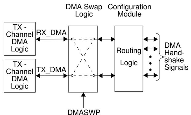
**FIGURE 5-26. DMA Control Signals Routing**
