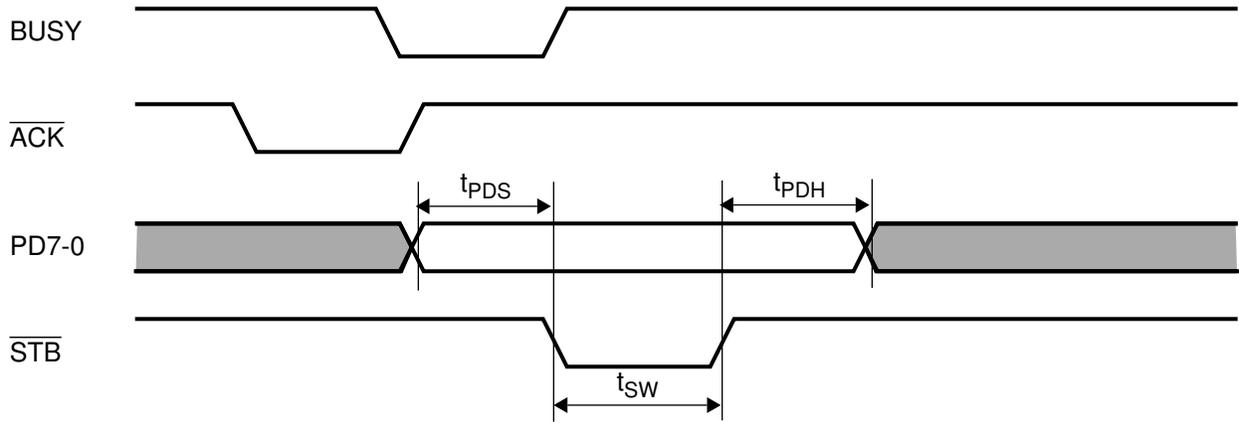
**FIGURE 8-24. Typical Parallel Port Data**
