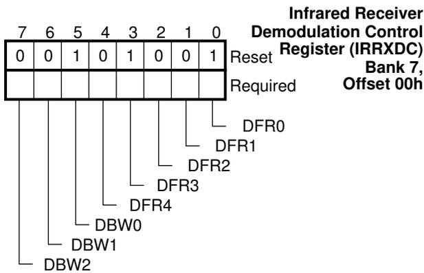
**FIGURE 5-50. IRRXDC Register Bitmap**
