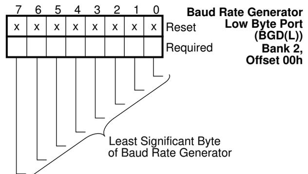
**FIGURE 5-23. BGD(L) Register Bitmap**
