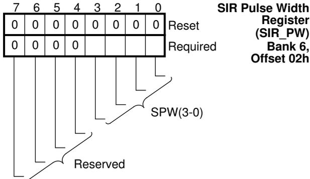
**FIGURE 5-48. SIR\_PW Register Bitmap**
