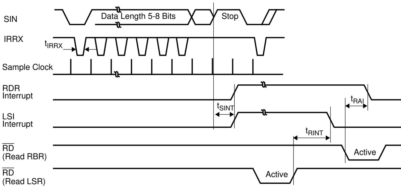
FIGURE 8-10. SIR Receiver Timing
