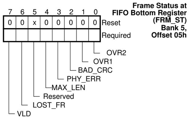
**FIGURE 5-43. FRM\_ST Register Bitmap**
