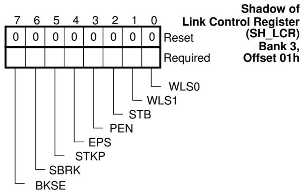
**FIGURE 5-31. SH\_LCR Register Bitmap**
