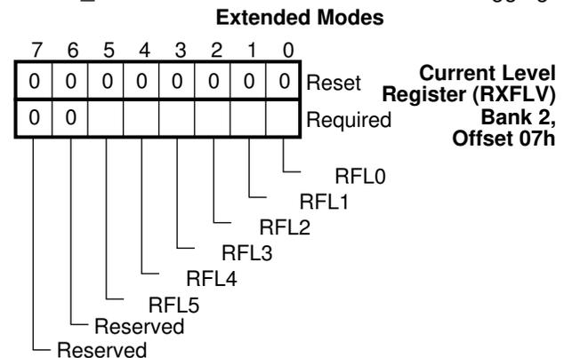
**FIGURE 5-29. RXFLV Register Bitmap**
