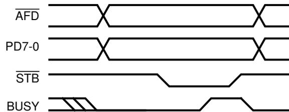
FIGURE 4-28. ECP Forward Write Cycle
