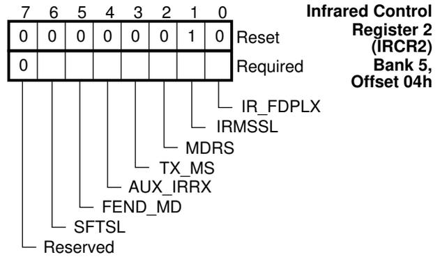
**FIGURE 5-42. IRCR2 Register Bitmap**
