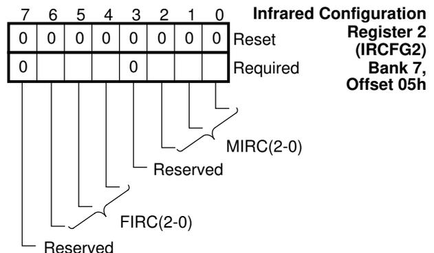
**FIGURE 5-54. IRCFG2 Register Bitmap**
