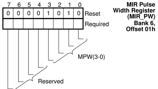
**FIGURE 5-47. MIR\_PW Register Bitmap**
