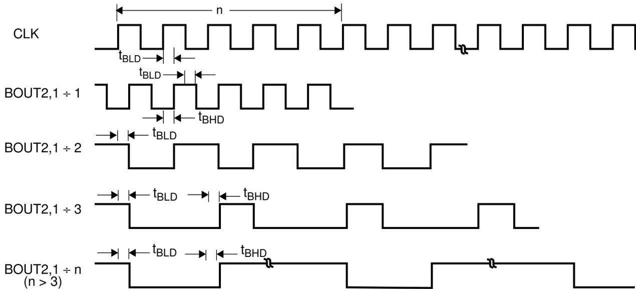
**FIGURE 8-7. Baud Output Timing**
