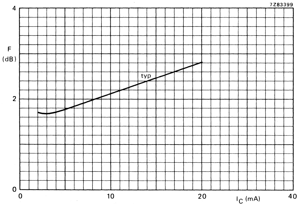
Fig. 9 V_{CE} = 10\text{ V} ; f = 800\text{ MHz} ; Z_S = \text{optimum} ; T_{\text{amb}} = 25\text{ }^\circ\text{C} ; typical values.
