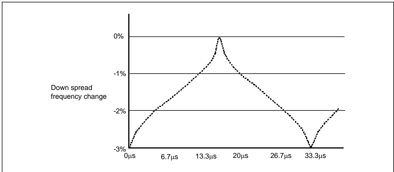
Analysis was done to show that, with a PLL bandwidth of 100x the modulation frequency and a phase angle << 0.1 degrees, tracking skew should be manageable. For the 405GP the tracking skew for up to a -3% variation in the SysClk frequency modulated at 30 kHz ranges from -77.5 to -185 ps depending on the VCO frequency. Tracking skew in pico seconds can be determined using the following formula.
